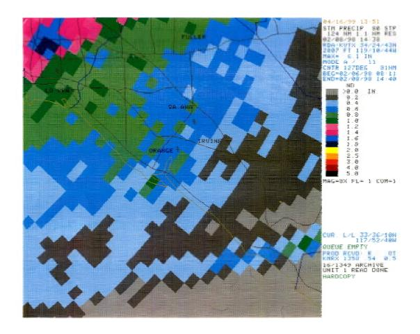
• Radar information is used to supplement rain gauge measurements in the evaluation of actual storm rainfalls during a particular storm event. The rain gauge data is used to calibrate the spatial distribution of rainfall estimated by radar. Radar data is used to describe what occurs between rain gauges.
